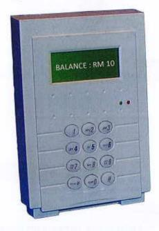
Green LED blinking – device reading card's information
